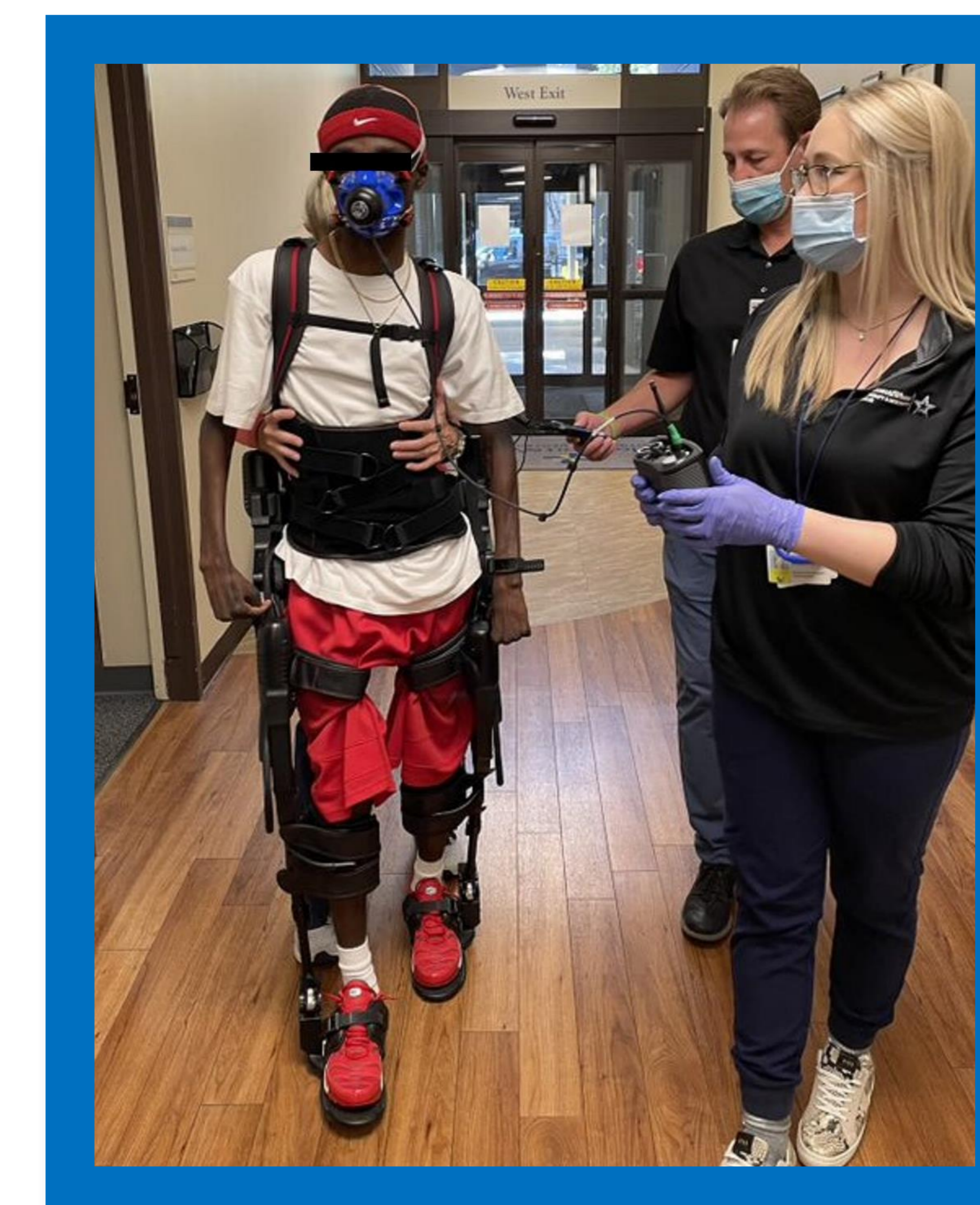
Figure 1. Utilization of a portable metabolic system to assess exercise intensity during OEGT in a patient with chronic tetraplegia
